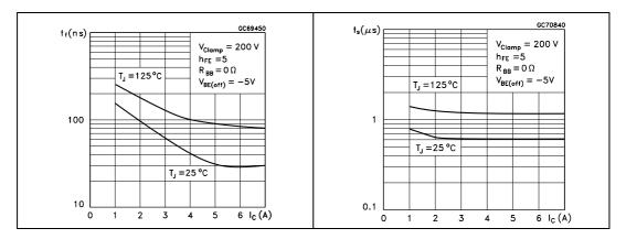
Figure 10. Resistive load fall time
